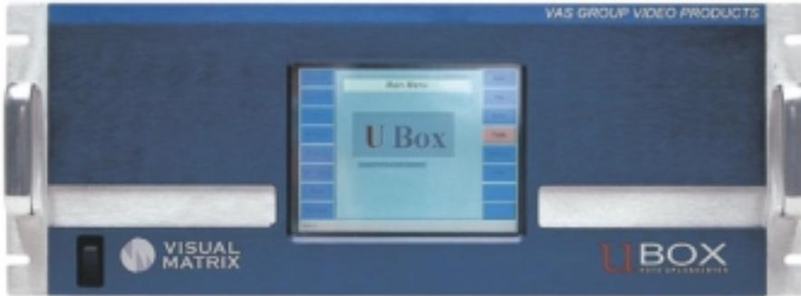
The UBox is a high quality HDTV upconverter that converts serial digital video (525 or 625) to digital television 480p, 720p and 1080 standards. The UBox has an extensive list of standard features including complete aspect ratio controls, advanced image enhancement filters and a film mode for improved upconversion of film sourced video.
